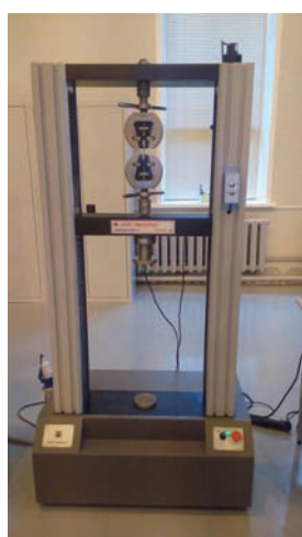
Fig. 3: Universal testing machine, IR 5082-5
